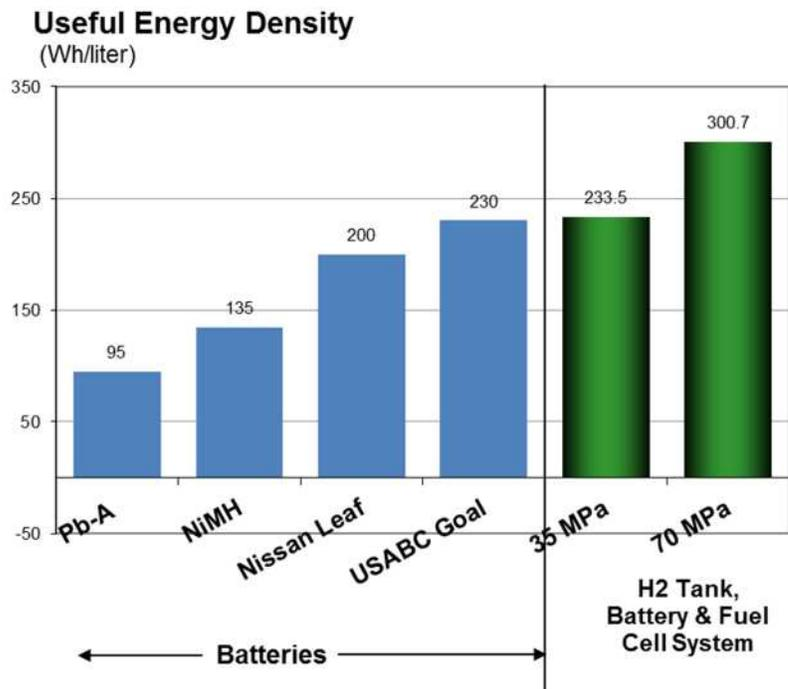
Figure 2 Useful Energy density (energy per unit volume--Large is good!) for batteries and for hydrogen/fuel cell systems
