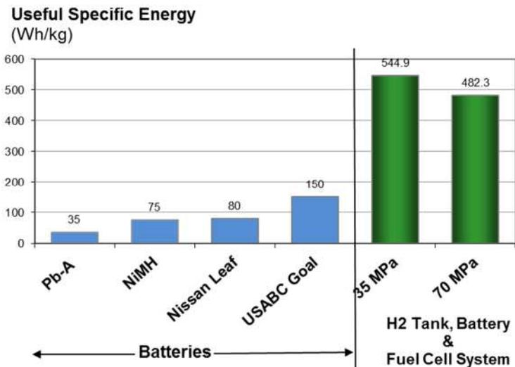
Figure 1. Useful specific energy (stored energy per unit mass—large is good!) for batteries and hydrogen/fuel cell systems
