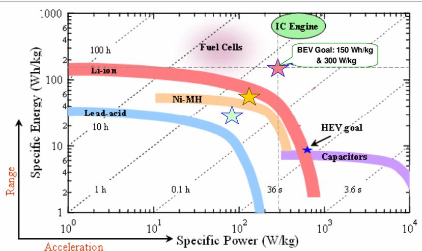
**Figure 7. Specific Energy vs. Specific Power for battery technologies from Kromer and Heywood (MIT) [6]; star symbols indicate the battery parameters used in this study that are all more optimistic than current battery performance**
