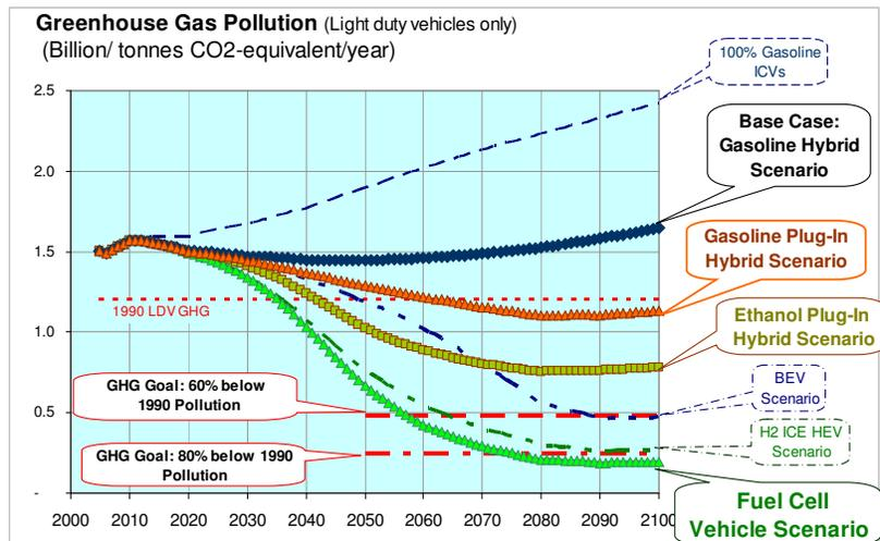
**Figure 1. Projected greenhouse gases for different alternative vehicle scenarios over the 21<sup>st</sup> century for the US light duty vehicle fleet, assuming that both the electrical grid and hydrogen production reduce their carbon footprints over time. The fuel cell electric vehicle and battery electric vehicle scenarios include gasoline ICEVs, HEVs and ethanol PHEVs in the mix (BEV= battery electric vehicle; H2 ICE HEV = hydrogen internal combustion engine hybrid electric vehicle)**
