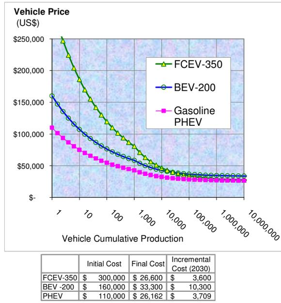
Figure 15. Estimated cost of alternative vehicles as a function of cumulative production volume
