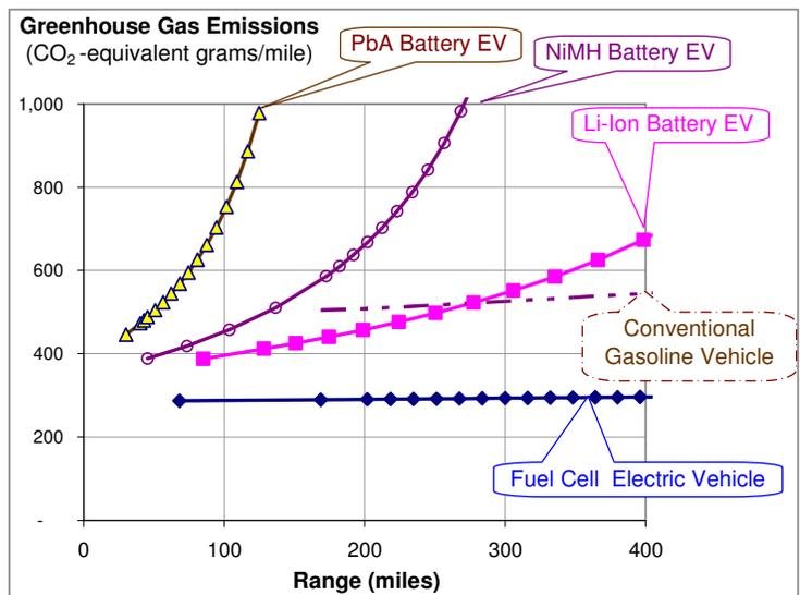
**Figure 8. Estimated greenhouse gas emissions for battery EVs and fuel cell EVs, using existing average US marginal grid mix for electricity and assuming that all hydrogen is made from natural gas**
