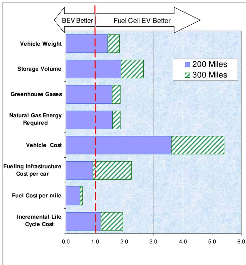
**Figure 12. Ratios of battery EV parameter divided by fuel cell EV parameter (Value greater than one favors the fuel cell EV)**
